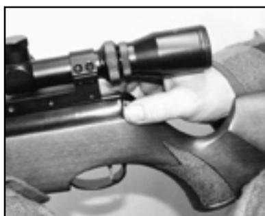
RELEASE THE SAFETY CATCH BY PUSHING THE BUTTON IN FULLY. THE RIFLE IS NOW READY TO FIRE. THE SAFETY CATCH CANNOT BE RE-ENGAGED WITHOUT RE-COCKING THE RIFLE SO DO NOT RELEASE THE SAFETY CATCH BEFORE YOU NEED TO.
