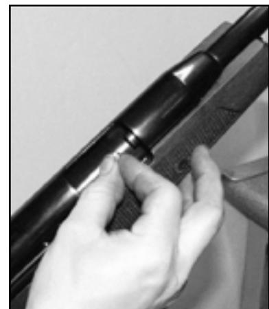
TO CLOSE THE COCKING ARM IT IS NECESSARY TO DEPRESS THE FRONT END OF THE SAFETY LOCK AND KEEP IT DEPRESSED UNTIL THE COCKING ARM IS FULLY CLOSED. ENSURE THAT THE IDENT BALL IS LOCATED IN THE IDENT. SERIOUS DAMAGE WILL RESULT IF THE RIFLE IS FIRED WITH THE COCKING ARM PARTLY OPEN.
