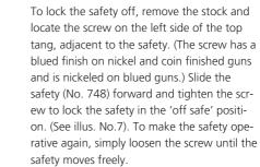
LOCK THE SAFETY IN THE 'OFF' POSITION ONLY WHEN SHOOTING CLAY TARGETS UNDER CONTROLLED CONDITIONS! Make the safety operative for ALL other shooting.
