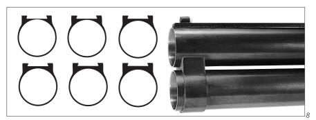
The point of impact of the bottom barrel of the K-80 and K-20 can be raised or lowered in relation to that of the top barrel simply by changing the front barrel hanger No. 606. The hangers have dovetails of varying width which change the height of the bottom barrel. (See illus. No. 8). If you wish to have the
